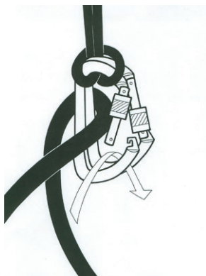
5a Clipping the Garda knot
